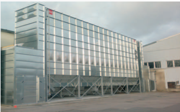
Line filter with reverse-air cleaning
